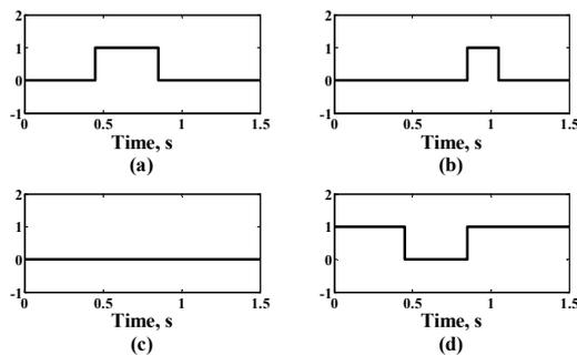
Figure 6. Logic signals when the line breaker is in maintenance. (a) Fault simulated. (b) Auto-reclose signal. (c) Line breaker position. (d) Middle breaker position
