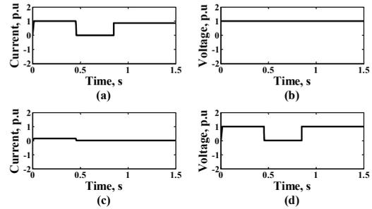
Figure 5. Currents and voltages for the normal operation (a) Current flow through 152L. (b) Voltage at BUS A. (c) Current flow through 152M. (d) Voltage at 152M.
