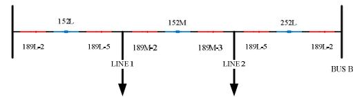
Figure 2. Line diagram for a section of breaker-and-a-half scheme
