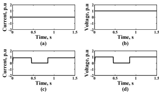
Figure 7. Currents and voltages when the line breaker is in maintenance (a) Current flow through 152L. (b) Voltage at Bus A. (c) Current flow through 152M. (d) Voltage at 152M.
