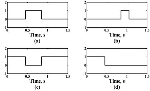
Figure 4. Logic signals when the line breaker is operating. (a) Fault simulated. (b) Auto-reclose signal. (c) 152L breaker position. (d) 152M breaker position.
