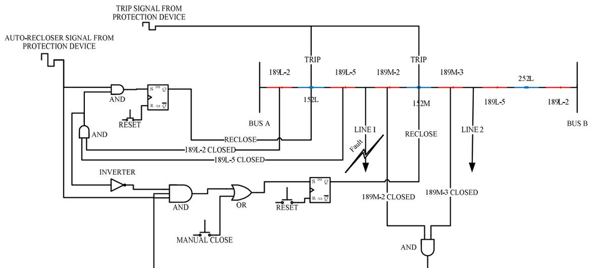
Figure 3. Line diagram for a section of breaker-and-a-half scheme
