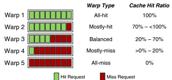
Figure 3: Warp type categorization based on the shared cache hit ratios. Hit ratio values are empirically chosen. Reproduced from [6].
